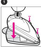
Attach carpet glide by placing unit under "tabs" and gently pushing down into place.
